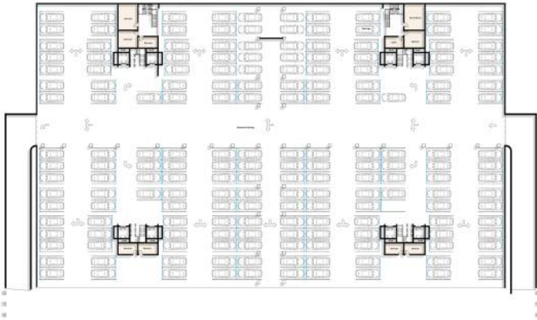
Basement parking plan — 180 bays, circulation and core
